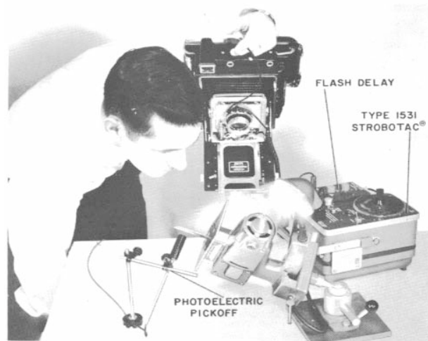
Figure 2.3. Stroboscope, Flash Delay, and Photoelectric Pickoff used for high-speed photography.
